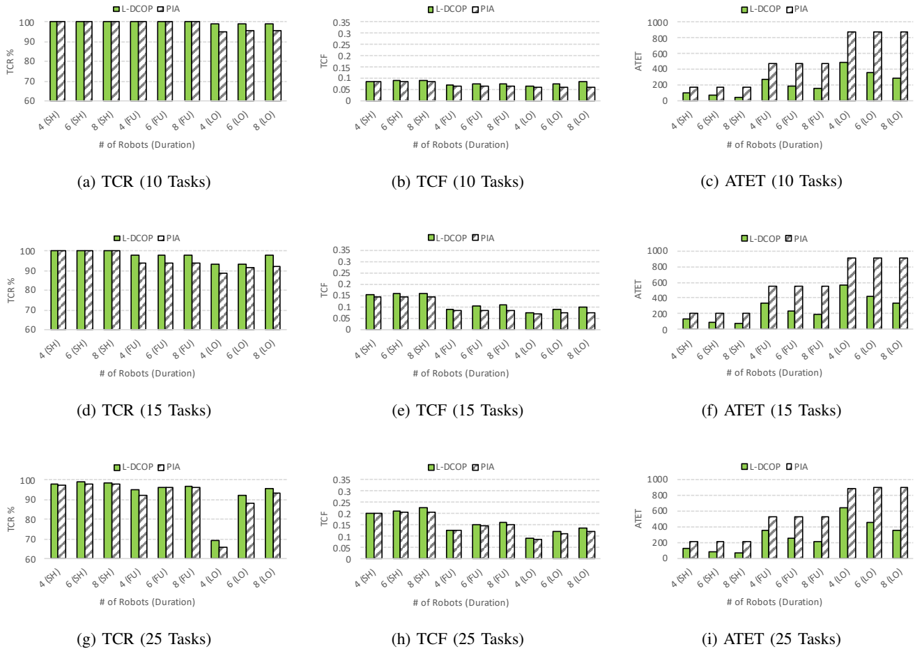
Fig. 6: Results for tasks with an EST within the first 50% of the scheduling time frame averaged over 25 randomly generated precedence graphs. Task duration: SH = [100, 300], LO = [800, 1000], and FU = [100, 1000].
