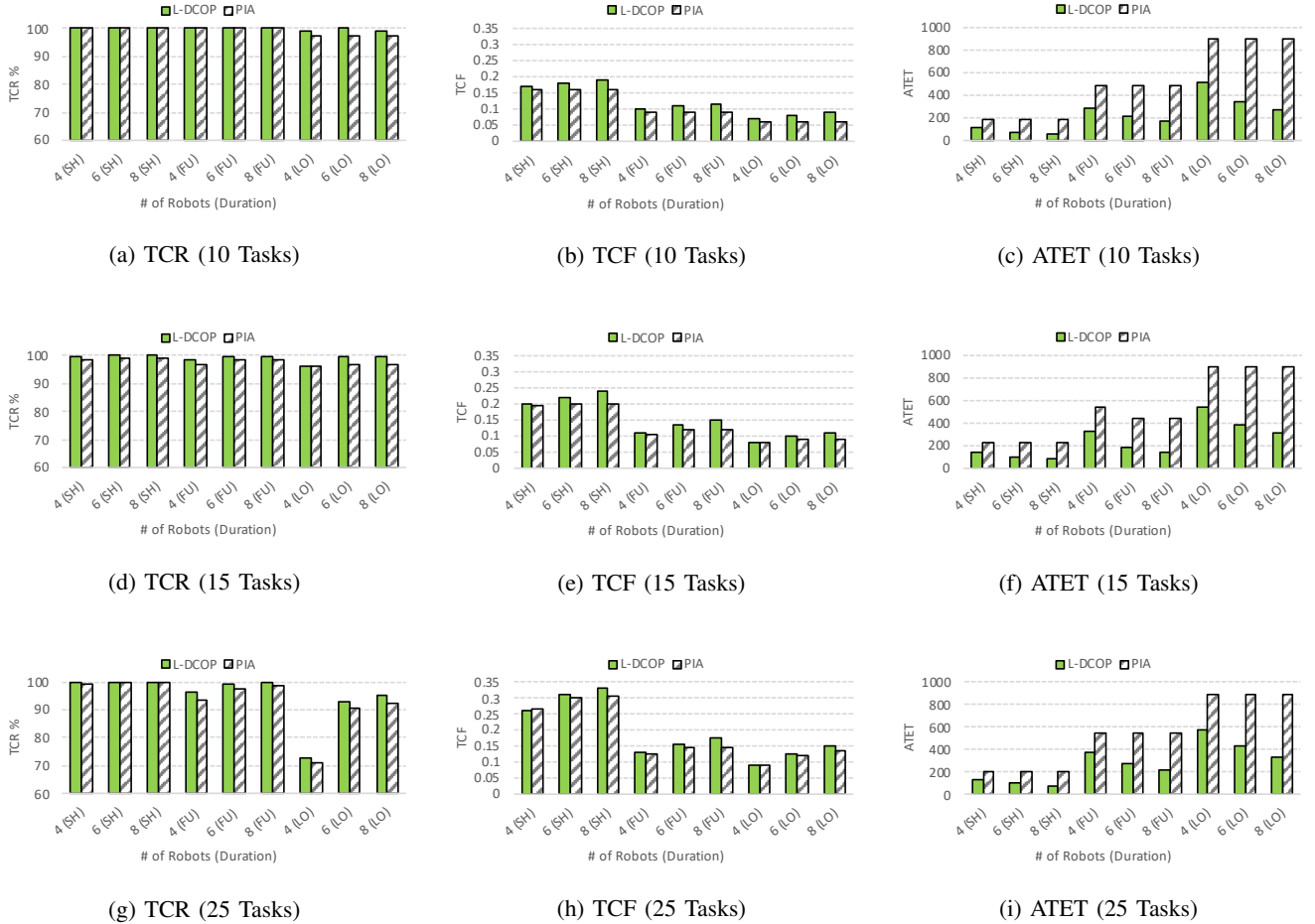
Fig. 5: Results for tasks with an EST within the first 25% of the scheduling time frame averaged over 25 randomly generated precedence graphs. Task duration: SH = [100, 300], LO = [800, 1000], and FU = [100, 1000].
